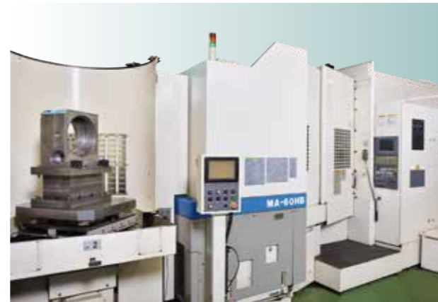
Adopting OKUMA MA-60HB HMC for Housing machining, the parallelism and perpendicularity in boring machining can be reached 0.005mm in between spindle hole and center hole of worm shaft.
